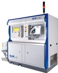
The Selective Laser Melting Machine SLM 280 2.0 provides a 280 x 280 x 365 mm<sup>3</sup> build envelope and a patented multi-beam technology. Available in several configurations, providing single optics (1x 400W or 1x 700W), dual optics (1x 700W and 1x 1000W) and twin optics (2x 400W or 2x 700W). Depending on how
