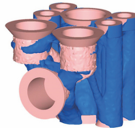
Figure 2: Interpretation and remesh of topology optimization results
