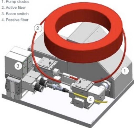
The diode laser with 8 mm-mrad is a technical enhancement of the existing LDF series. Starting from a standard diode laser, the laser beam, at medium beam quality is first focused into an active fiber. This improves the **laser beam quality** by conversion technology so that a beam quality better than **8 mm-mrad** is attained at the active fiber outlet.
